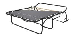
One -piece, heavy gauge steel construction featuring perfectly spaced comfort supports to provide a level mattress foundation to eliminate bar in back discomfort. Anti-tilt safety feature to keep mech in contact with the floor when open. One-piece tubular legs for stability and strength.
